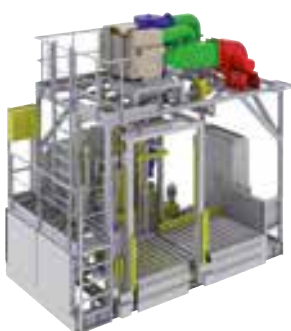
3D model of mobile DeDuster® installed on bagging machine
