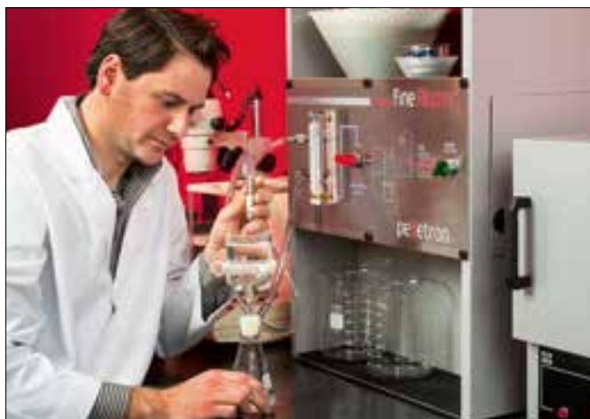
FineAlyzer®, Pelletron Corporation's wet test device
