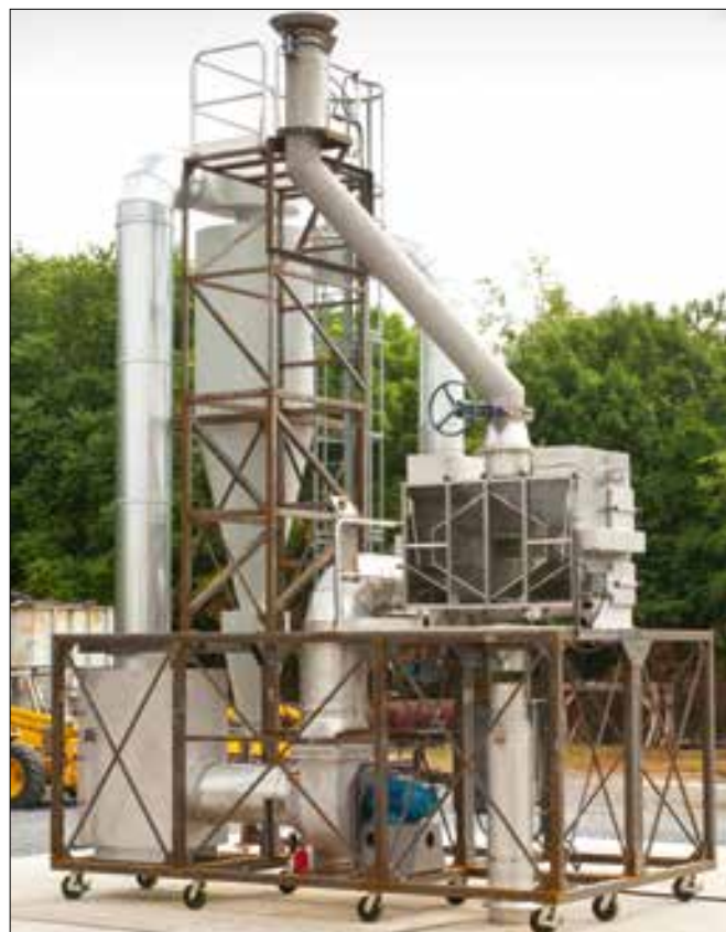
Mobile DeDuster® for 60 t/h capacity preassembled in the shop
